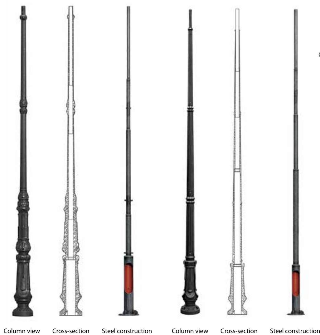
An example of the construction of the pole S-40W
