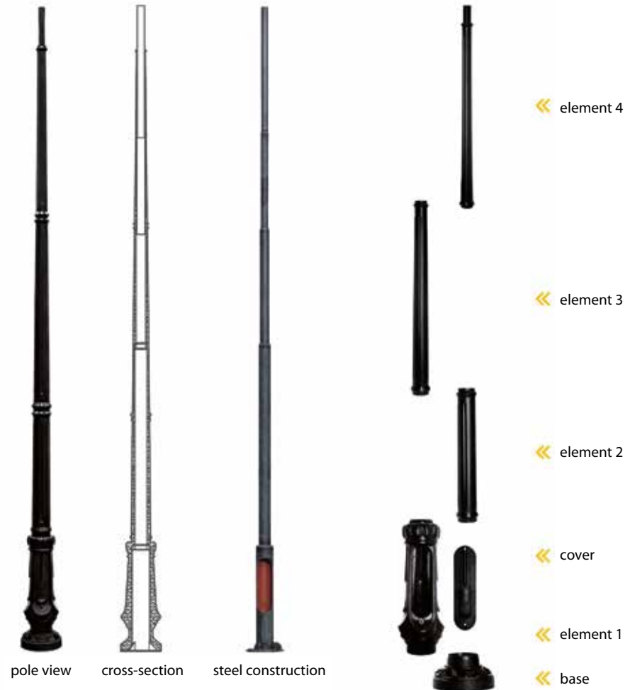
Example of the pole construction SM-1W/E
